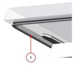
Figure 20: Replacing the lid gasket
