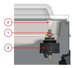
Figure 2: Overview of the seal system
