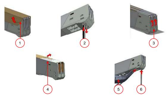
Figure 18: Replacing the sealing wire
