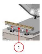
Figure 17: Removing the seal bar
