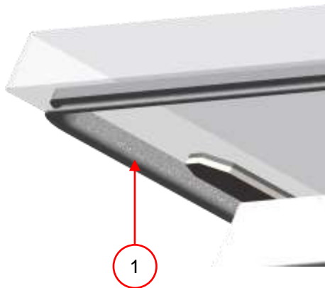
Figure 15: Replacing the lid gasket
