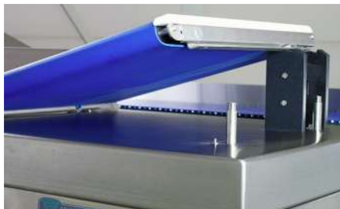
Figure 14: Use the provided stand to hold the conveyor belt in upper position for cleaning purposes.
